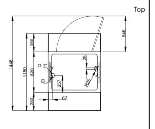
Electric Supply voltage: 322021 (F02H2AW04S) 220-240 V/1N ph/50/60 Hz Electrical power max.: 2.32 kW Water: Drain line size: 3/4" **Key Information:** N° of doors: External dimensions, Width: 800 mm External dimensions, Depth: 1180 mm External dimensions, Height: 1304 mm Net weight: 97.5 kg Shipping height: 1334 mm
